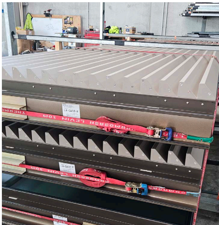
Prefabricated Thermosash Thermoplank unitised rainscreen, packed for transport to site.
