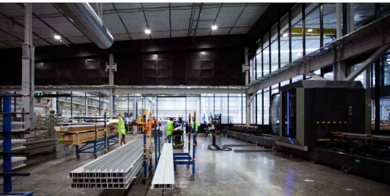
Thermosash Henderson, Auckland CNC machining centre enclosed in a Thermosash PW1000 acoustic curtainwall.
